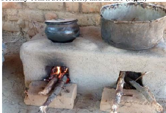
Figure 3 The Changu Changu Moto improved cook stove, recently constructed (left) and in use (right)
